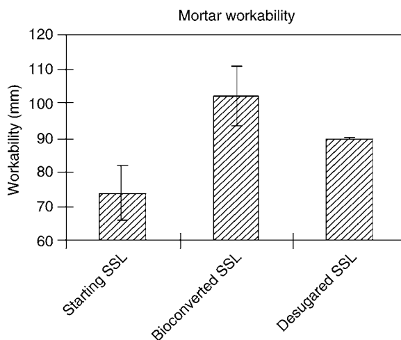
Fig. 11. Mortar workability test results of the bioconverted hardwood (birch) spent sulfite liquor (SSL) along with the starting SSL and the corresponding desugared SSL. The cement/sand/water ratio was 384/1350/230 ( w/c = 0.598 ). Dosage was fixed at 0.1% on cement. Average of duplicate tests and the bars in the chart show the range of the data.
